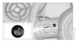
nd This symbol on the Control Display and an acoustic signal indicate that the voice activation system is ready to receive spoken commands.
