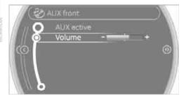
Turn MINI joystick until the desired volume is set and then press the MINI joystick.
