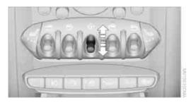
The switch locks or unlocks the doors and liftgate when the doors are closed, but the antitheft system is not activated. The fuel filler flap remains unlocked\*.
