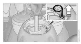
Insert extractor hook 1 into the loop on the passenger's side.
