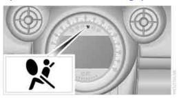
As of radio readiness, page 46, the warning lamp lights up briefly to indicate that the entire airbag system and the belt tensioners are operational.
