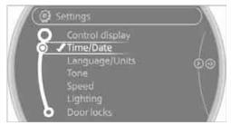
Turn the MINI joystick until "Time:" is selected, and press the MINI joystick.
