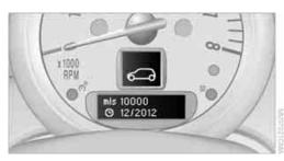
The remaining driving distance and the date of the next scheduled service are briefly displayed immediately after you start the engine or switch on the ignition.
