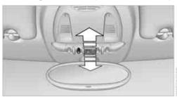
To switch the interior lamps on/off.
