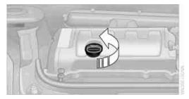
Do not add the maximum quantity of 1 US quart/1 liter of engine oil until the oil level has dropped to just above the lower mark on the dipstick, page 199.
