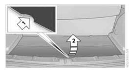
Lift up load floor behind and fold forwards, arrow 2.
