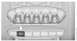
Press the button to switch the lamps on and off.
