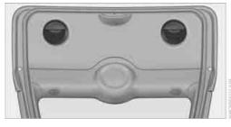
The handle recesses on the interior trim panel of the liftgate make it easier to pull it down.
