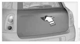
Press the top side of the MINI emblem, arrow, or Press the button on the remote control for approx. 1 second and then release it. The lift-qate is unlocked.
