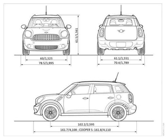
All dimensions in inches/mm. Minimum turning radius dia.: 38.1 ft/11.6 m. Information after the semicolon: different values for MINI Cooper S.
