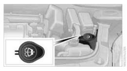
Fill with water and, if required, with a washer antifreeze, according to manufacturer's recommendations.
