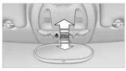
To switch the interior lamps on/off.
