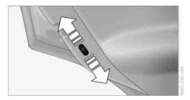
Slide down the safety lever on the rear doors. The door can now be opened from the outside only.
