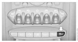
Press the button until the DSC OFF indicator light on the speedometer is on and DSC OFF is displayed on the tachometer. DSC is deactivated. Stabilizing and propulsion promoting actions are no longer executed.
