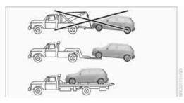
Have the MINI Countryman transported by a tow truck with a so-called lift bar or on a flat bed.
