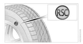
The symbol identifying run-flat tires is a circle with the letters RSC on the sidewall.
