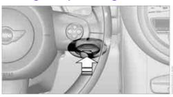
Insert the key all the way into the ignition lock. Radio readiness Individual electrical consumers can operate.
