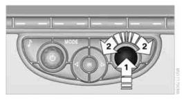
Press the knob, arrow 1, to confirm a highlighted function.
