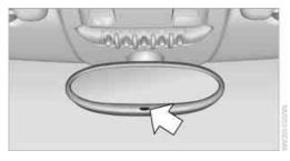
It is controlled by two photosensors:
