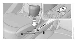
First insert the cupholder into the front mounts 4 and then snap it into the rear mounts 5.
