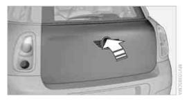
Press the top side of the MINI emblem, arrow, or Press the button on the remote control for approx. 1 second and then release it. The liftgate is unlocked.
