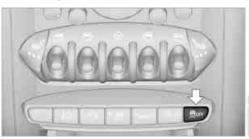
Press the button; the indicator light DSC OFF on the speedometer comes on and TRACTION is displayed on the tachometer.
