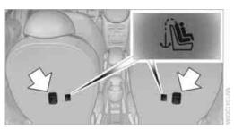
There are two additional anchors for child restraint systems with tether straps, arrows.
