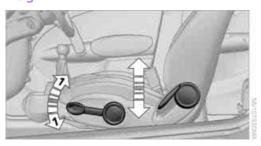
Pull up or push down the lever repeatedly, arrows 1, until the desired height is reached.
