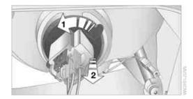
Push on the catch, arrow 1, and disconnect the connector, arrow 2.
