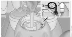
Insert extractor hook 1 into the loop on the passenger's side.
