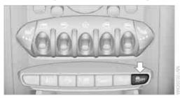
Press the button for at least 3 seconds; the indicator light DSC OFF on the speedometer comes on and DSC OFF is displayed on the tachometer. The Dynamic Traction Control DTC and Dynamic Stability Control DSC are both deactivated. There will be no more stabilizing interventions.
