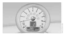
Never operate the engine with the needle in the red overspeed zone of the gauge. In this range, the fuel supply is interrupted to protect the engine.
