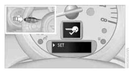
Press and hold the button until the display changes. 6. Briefly press the button repeatedly until the display shows the illustrated symbol, arrow.
