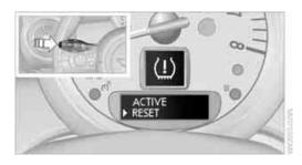
Press and hold the button until "RESETTING" is displayed.
