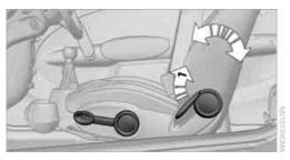
Pull lever, arrow 1, and apply weight to or remove weight from the backrest as needed.
