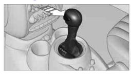
Press the button on the front of the selector lever, arrow.
