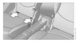
The mounts for the lower LATCH anchors are located at the points indicated by the arrows.
