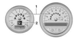
Indicator and warning lamps can light up in various combinations and colors in indicator area 1 or 2.
