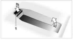
Insert the snap-in adapter at the front, arrow 1, and press downward, arrow 2, until it clicks into place.
