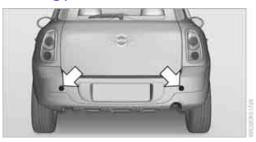
The mounting points are located under the covers in the bumper.
